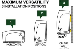
Horizontal, vertical or wall mounted, E.sybox can be all the control of the contr installed virtually anywhere inside or outside the home.
