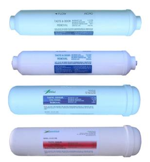
XIN10 and LCL10 Coconut shell Granular Activated Carbon (GAC) remove chlorine, organics, colour, objectionable tastes and odour from water. Offered in ¼" female threaded and ¼" QC (quick connect) style ends, these self-contained filters are installed in-line, eliminating the need for an additional housing.
