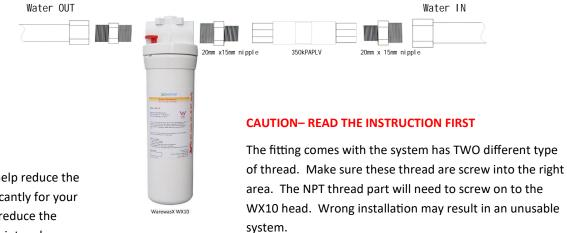
1. Tape the both NPT brass fitting ends and screw it onto the WX10 head.
