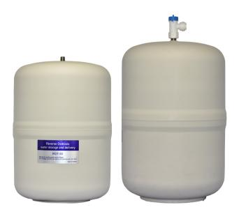
All Xsential reverse osmosis systems come with a storage tank. A pressurized storage tank for reverse osmosis product water is needed to deliver reverse osmosis water to the faucet or appliance using air pressure within the tank. Water is stored in a bladder within the tank vessel opposite pressurized air.
